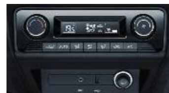
Climate control air conditioning
